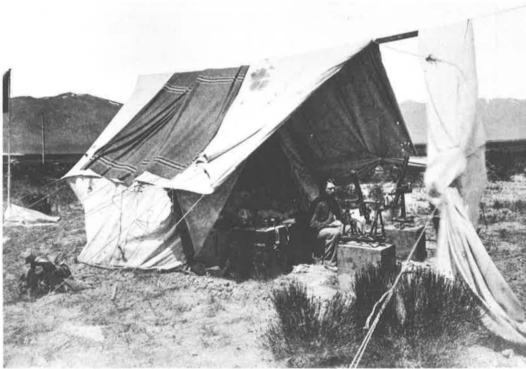
Figure 6. Topographer Allen Wilson at the King survey's "astronomical observatory" in the Ruby Valley, northeastern Nevada, August 1868. Wilson holds a chronometer and faces the zenith (at right) and meridian (at left) telescopes. The telegraph to Wilson's right connected to the "observatory," via the transcontinental line's relay at nearby Camp Ruby, with the Coast and Geodetic Survey's astronomical station at Salt Lake City. Photograph by O'Sullivan.
